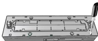
(Optionally take away the IP54-cover by loosening the 4 fixing screws) and remove the lamp. Now loose the top enclosure at the snap hooks by the help of a corresponding screw driver.
