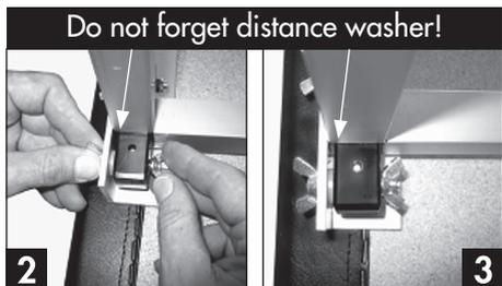
Secure everything with the wing nut and screw tight (2+3). Afterwards please tighten the wing screw with the self-locking nut again.
