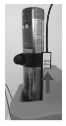
10- Set-up the line width by adjusting the height of the aerosol holder with the buttonscrew on the back of the sliding bar.
