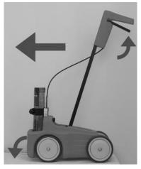
11- Swing the marking target into position, line-up on the chalk line or the existing line, press on the trigger and start your marking. Your pace should be at 30 seconds for 10 meters.
