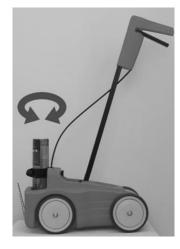
8- Pivot the Tracing PRO aerosol can 90° on both the right and the left sides until you can hear the « Click » which assesses the proper set-up of the nozzle into the spray activation module.
